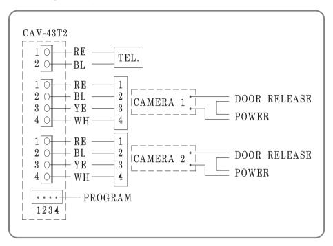
For better image quality when using UTP CABLE[CAT.5], connect the rest 4 lines to GND after connecting 4 lines with monitor and camera.
